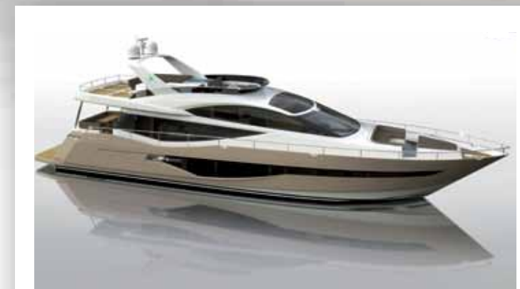
HULL SIDE WINDOWS AND GLASS PANEL ROOF
